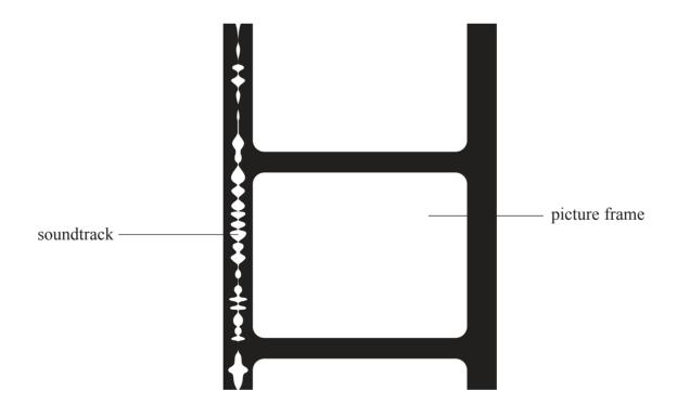
The film, including the soundtrack as shown, moves through a projector past a source of light. Light is detected by a phototube on the other side of the soundtrack. The changing current produced by the phototube circuit is converted to a sound signal with the same variation in amplitude and frequency as the original sound.
